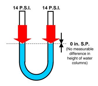
Water in an open U-Shaped Tube is level. Air pressure pushing down on it on both sides is <u>equal</u>. Static Pressure (S.P.) = 0 inches W.C.
